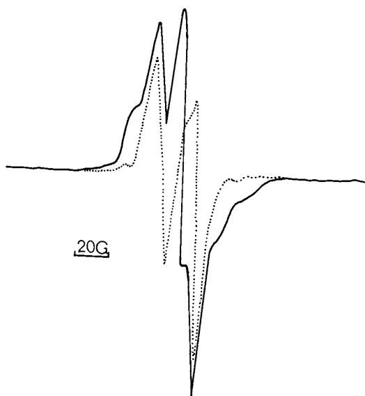
Figure 7. ESR spectra of carboxymethylcellulose irradiated with UV light of \lambda > 254 nm at 77 K for 60 min. Spectra were recorded at 77 K. Dotted line signal was obtained when sample was warmed to ambient temperature for 1 min.
